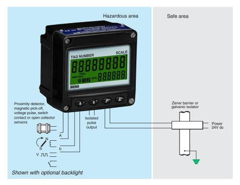
The BA384G is a two input, field mounting, intrinsically safe rate totaliser that can simultaneously display the total flow and rate of flow of either flowmeter, or the sum or difference of the two. The BA384G is easy to use and each input can be individually configured on-site to operate with flowmeters having a variety of pulse outputs. A slide-in scale card simplifies identification and international certification permits worldwide installation.
