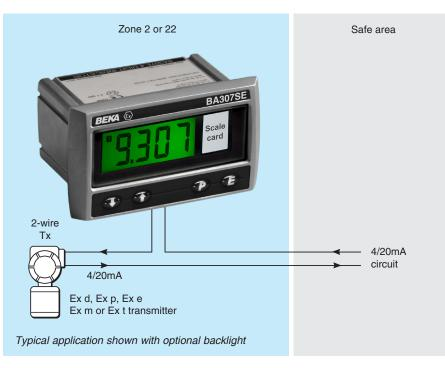
**The BA307SE** loop powered, panel mounting Indicator has a rugged stainless steel housing allowing it to be safely installed in an Ex e, Ex t or Ex pzc panel located in Zones 2 or 22 without the need for Zener barriers or galvanic isolators. The indicator has a full 4 digit display with guaranteed performance between -40 and +70°C. The scale card can easily be marked to show the units of measurement and can be fitted on-site without dismantling the instrument or removing it from the panel.
